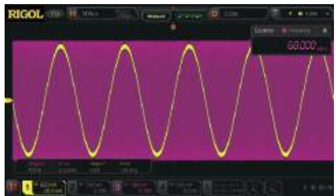
The ordinary 1 Mpts software measurement can no longer measure the accurate frequency of the high-frequency signal.
