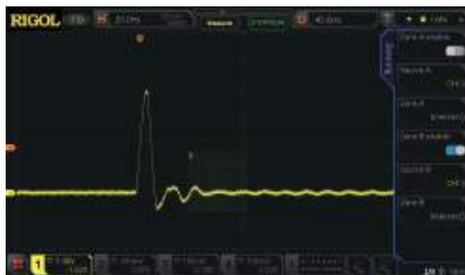
Quickly isolate the exceptional signal with Edge trigger and Zone trigger.
