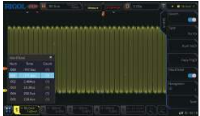
The search and navigation function can quickly search for the signals with exceptions and locate them accurately.
