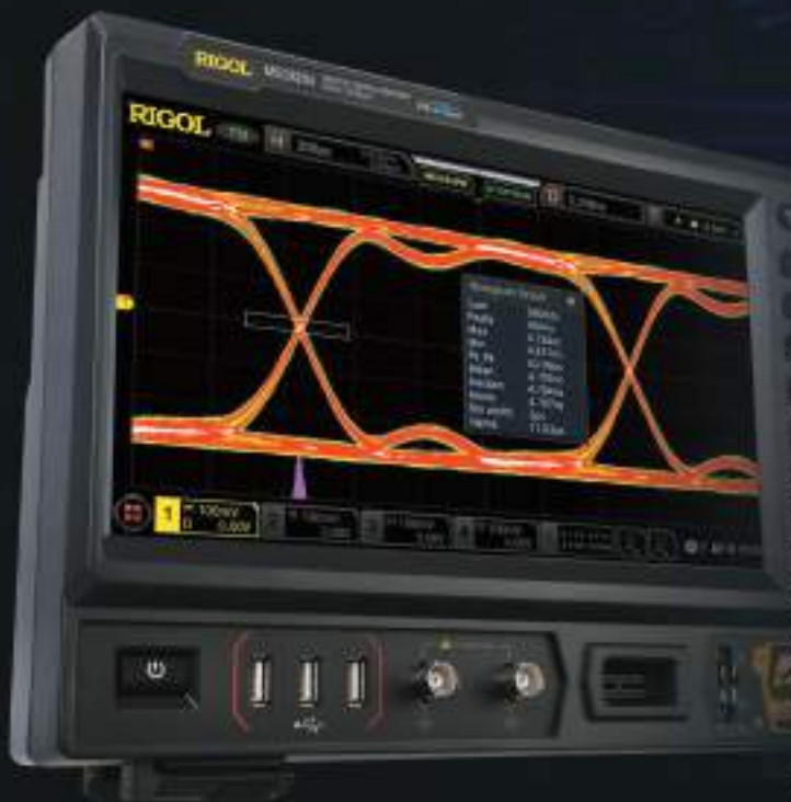
Perform eye measurement on the 622 Mb/s signal.
