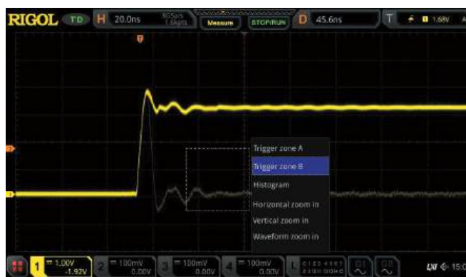
Draw a rectangle on the transient exception signal and select Trigger zone B.
