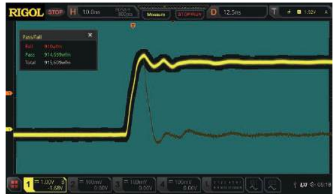
The Pass/Fail test function can quickly make statistics on the occurrence probability of the signal exceptions.
