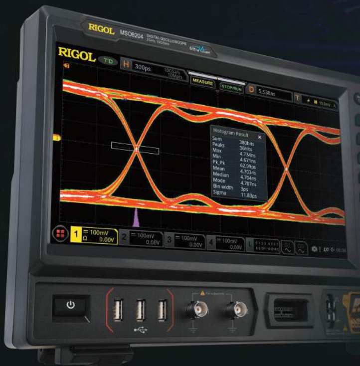
Perform eye measurement on the 622 Mb/s signal.
